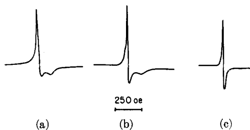
FIG. 6. The change of the shape of the ESR signal of Cr(V) during course of ethylene polymerization.
